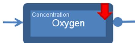
Fig. 2. A node in a MILA model, representing the trend of Oxygen Concentration Decreasing in a system.
